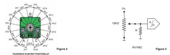
Connecting the collector terminal to the AD port of a microcontroller to feed the output voltage of said configuration will allow for the selection of 16 different functions.
