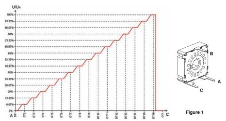
The detents are set to position and fix the wiper contact on the surface of each silver zone thus absorbing any mechanical play and printing tolerances. The electrical contact between the metal surface of the wiper and the silver area minimizes the contact resistance. The mechanical detents are evenly spread 22.5°±3° from each other along the circumference as it can be seen in the figure 2 drawing.
